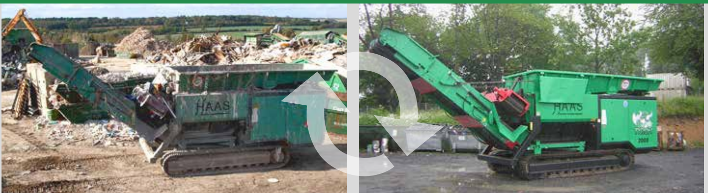
Photo comparison: HAAS TYRON with 15.000 operating hours before and after refurbishment.
