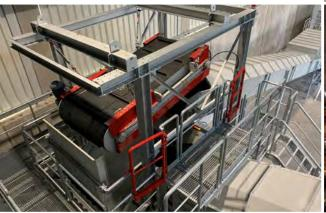
The ARTHOS shreds up to 40 tonnes of pre-shredded waste wood per hour to a size < 100 mm. The ballistic chute quarantees troublefree operation and therefore protects the hammermill, downtimes are minimised!
