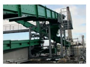
The processed chips are transported by a chain conveyor to another overband magnet, followed by an ECS, i.e. the ferrous and non-ferrous parts released in the hammermill are removed from the wood material flow. The chips, freed from foreign bodies, are fed into the following large flat screen, Type HPS 125. This screen separates the processed high quality chips into different fractions, such as 0-10, 10-30, 30-80 and > 80 mm, for example.
