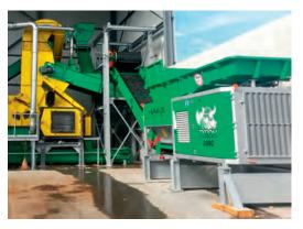
shredded and pre-cleaned waste wood to the heart of the plant, a HAAS hammermill with vertical infeed, which grinds the material into high quality chips. The tried and tested technology for the secondary shredding of biomass, waste wood, RDF, as well as plastic and PVC has consistently been developed further. Foreign bodies, such as hard plastic, ferrous -/ or non-ferrous material, etc., which can be transported into the hammermill together with the waste wood, in the past had to be removed
