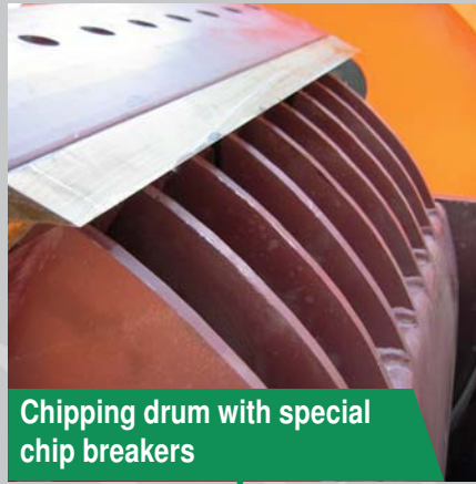
Rotor hood with wear protection plate
