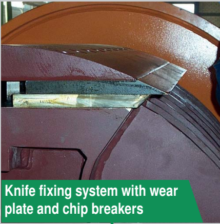
Chipping drum with special chip breakers
