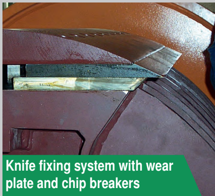
Chipping drum with special chip breakers
